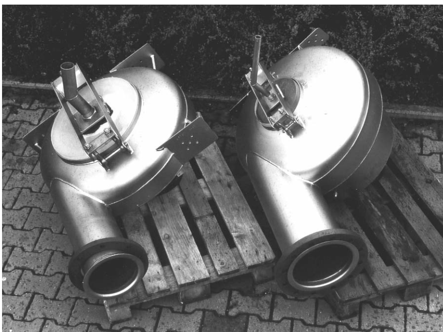
Bild 7: Two Vortex Flow Regulators form stainless steel, Model UFT-FluidCon. left: type SUT 30-4, DN 200, right: type SUT 45-3, DN 250.
